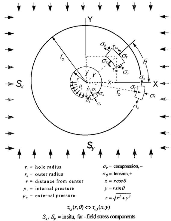
Figure 4. Stress distribution for unequal horizontal far-field in-situ stress state - linearly elastic, non-porous, isotropic system.
