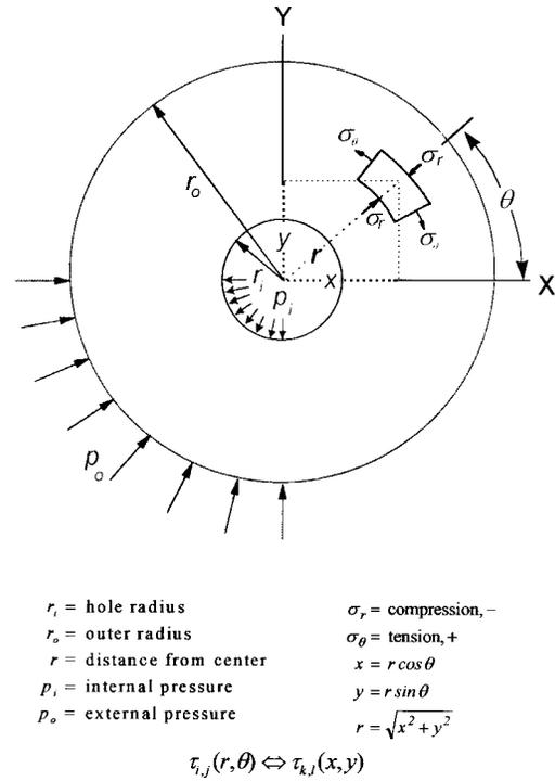
Figure 3. Stress distribution for equal horizontal far-field in-situ stress state - linearly elastic, non-porous, isotropic system.
