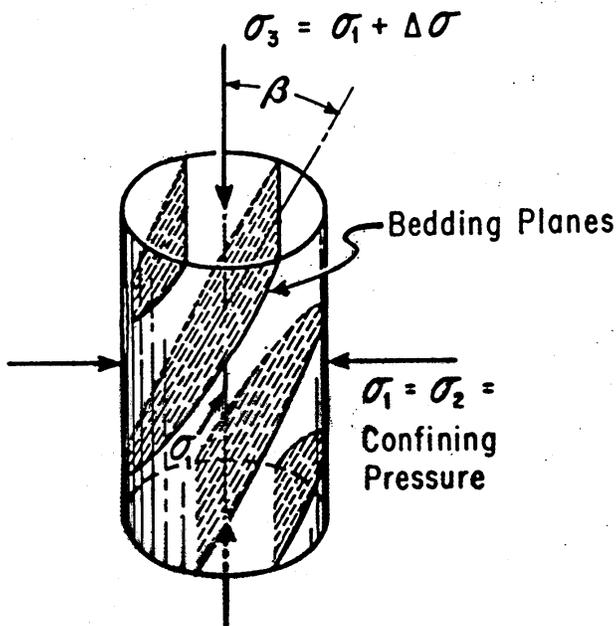
Figure 6. Bedding plane orientations for strength tests.
