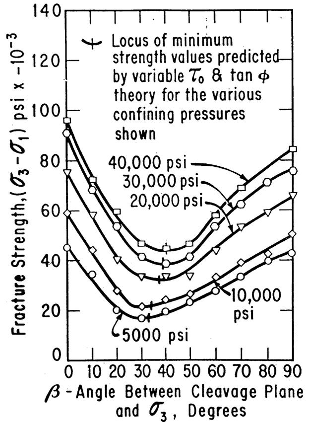
Figure 7. Fracture strength anisotropy due to bedding planes.
