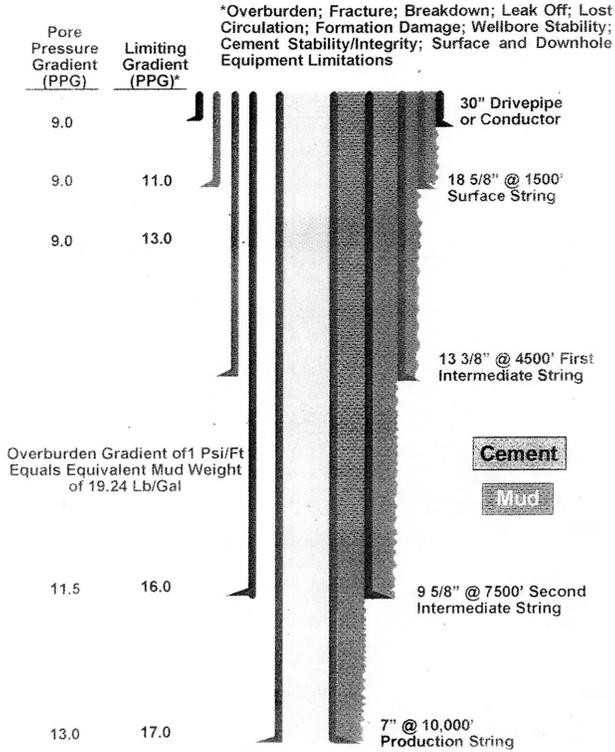
Figure 1. Example casing program.
