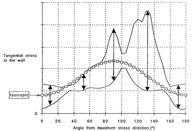
Figure 16. Tangential stresses on wellbore for isotropic and anisotropic rock, 3-D stress states.
