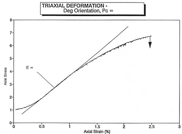
Figure 8. Stress, strain, and failure test on North Sea shale.
