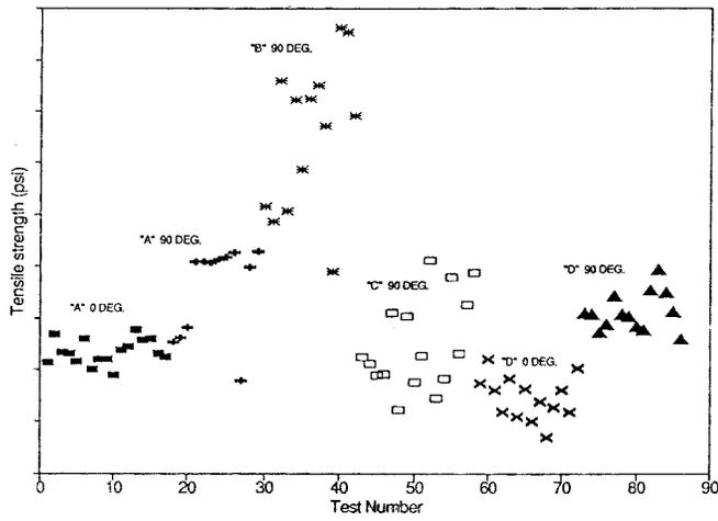
Figure 9. Anisotropic tensile strength of shales.
