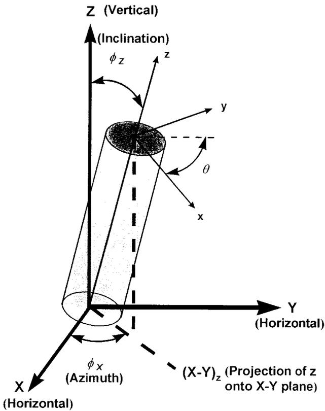
Figure 5. Far field and wellbore reference axes for inclined/horizontal wells.
