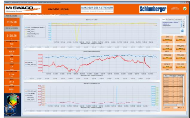
Fig. 4. Onshore SLB online viewer with Semi-automatic rheology, density and drilling parameters integration.
