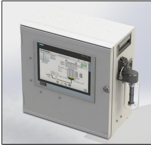
Fig. 1. Outside view of the Semi-automatic rheology and density device. The sample container is on the right side and the touchscreen at the front.
