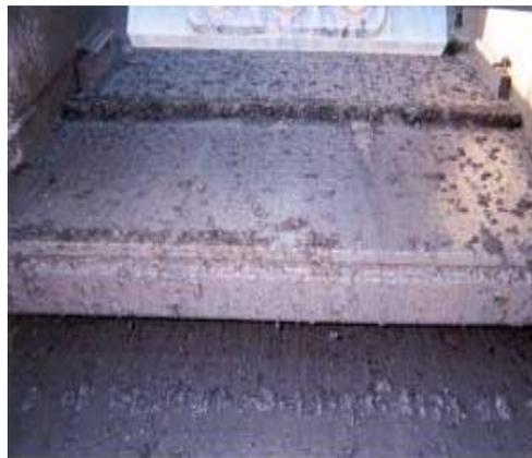
Fig. A8 - Typical cuttings shape and volume on the shaker through Atoka shale.
