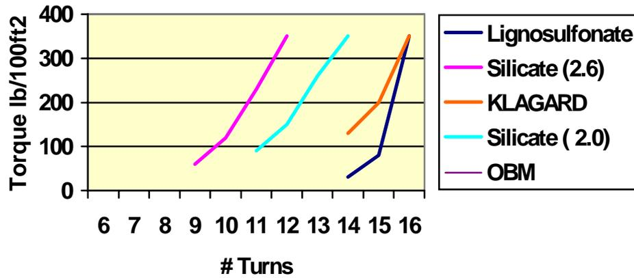
Fig. 4 - Bulk hardness test results.
