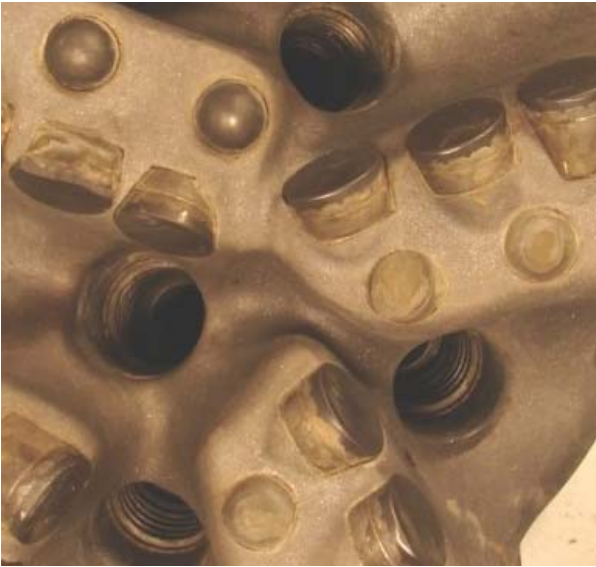
Figure 11: Test Bit with Different Material Inserts
