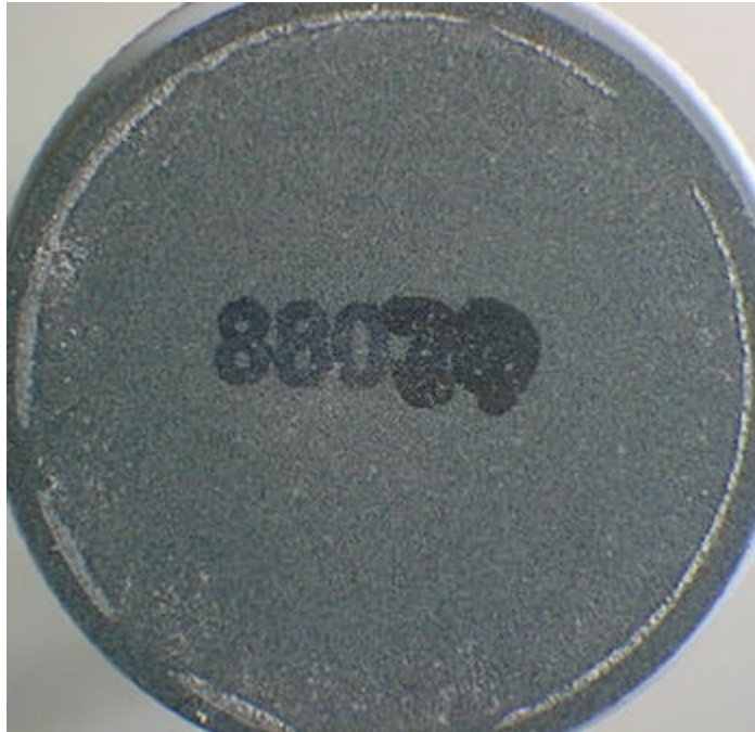
Fig. 2 - Filter cake from the 11.5 lb/gal NBRDF fluid in Table 12, Test #1 after acid treatment. Note that the residual cake is so thin that the disk type number is easy to read through the residual cake.
