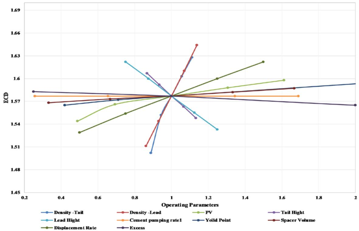
Figure 2: Cement design parameters sensitivity plot
