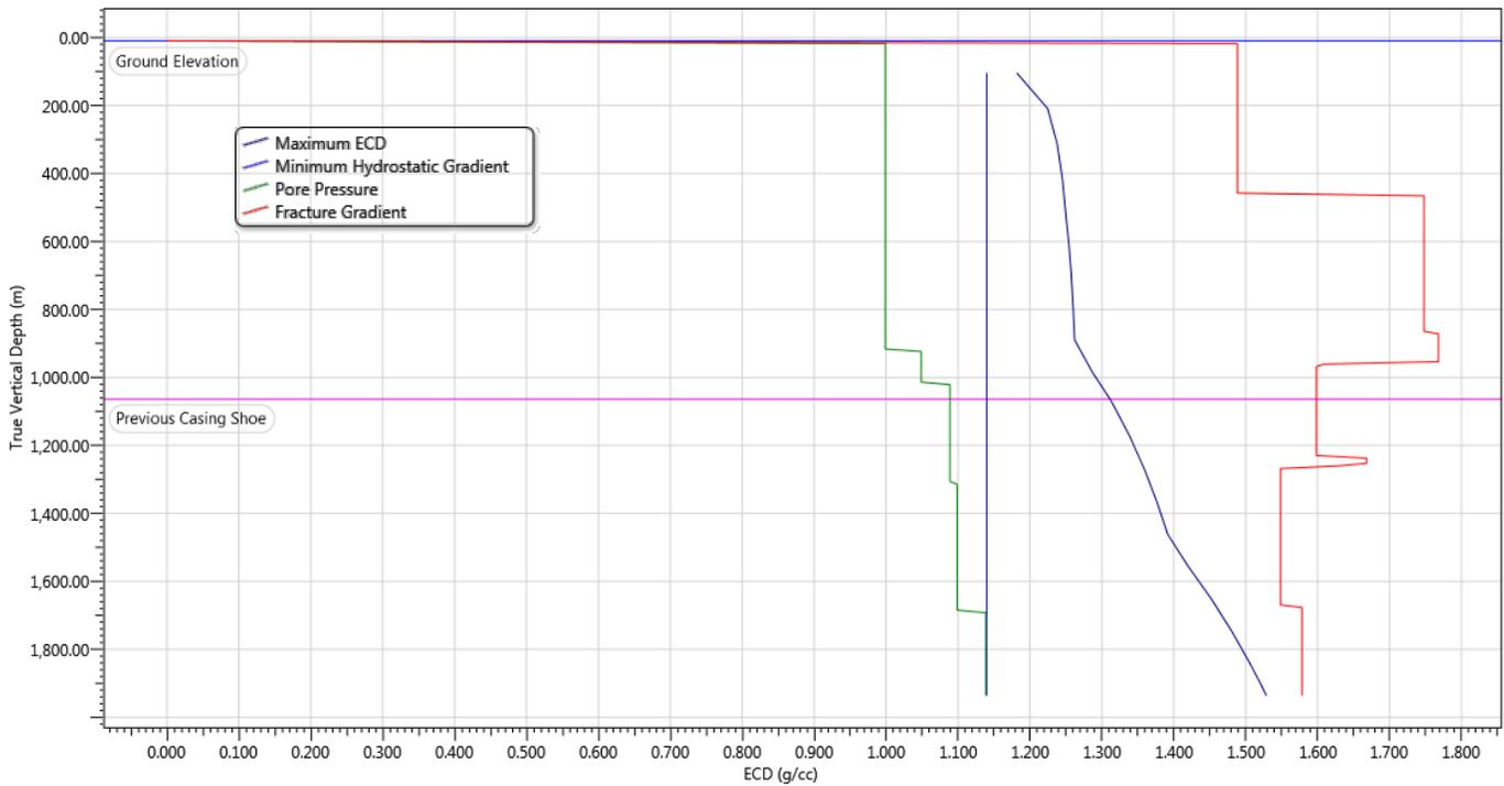
**Figure 9: The operation parameters for cement design when no losses is recorded**
