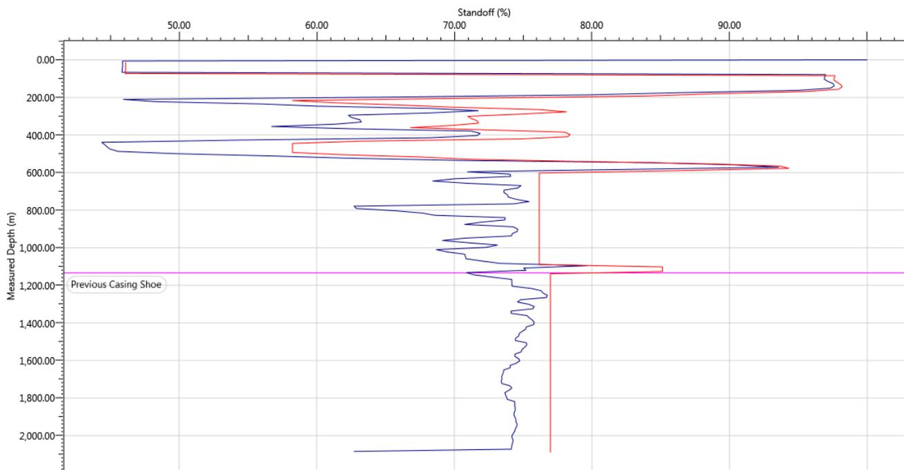
Figure 4: Optimum casing standoff
