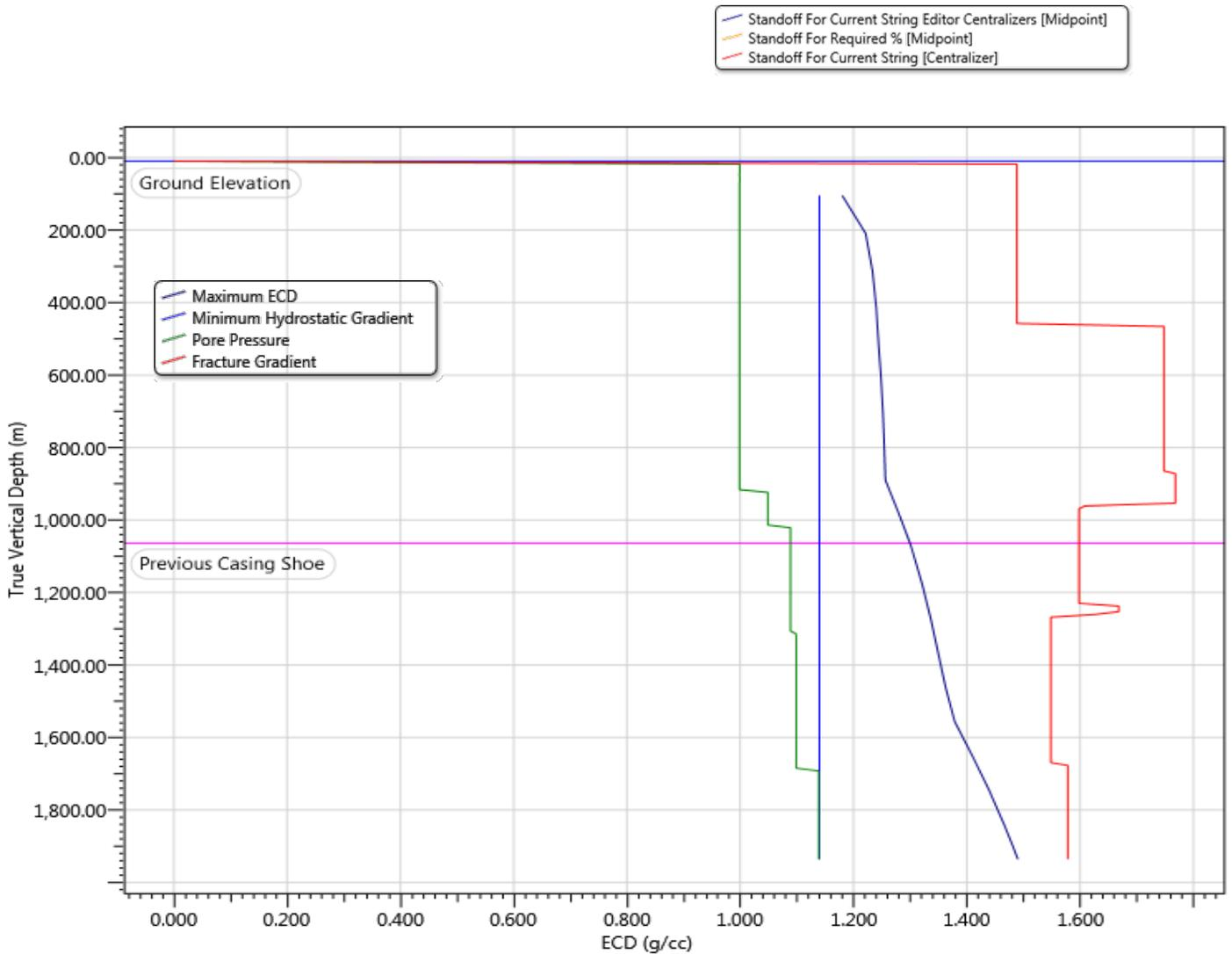
**Figure 5: The operation parameters for cement design when partial losses is recorded**
