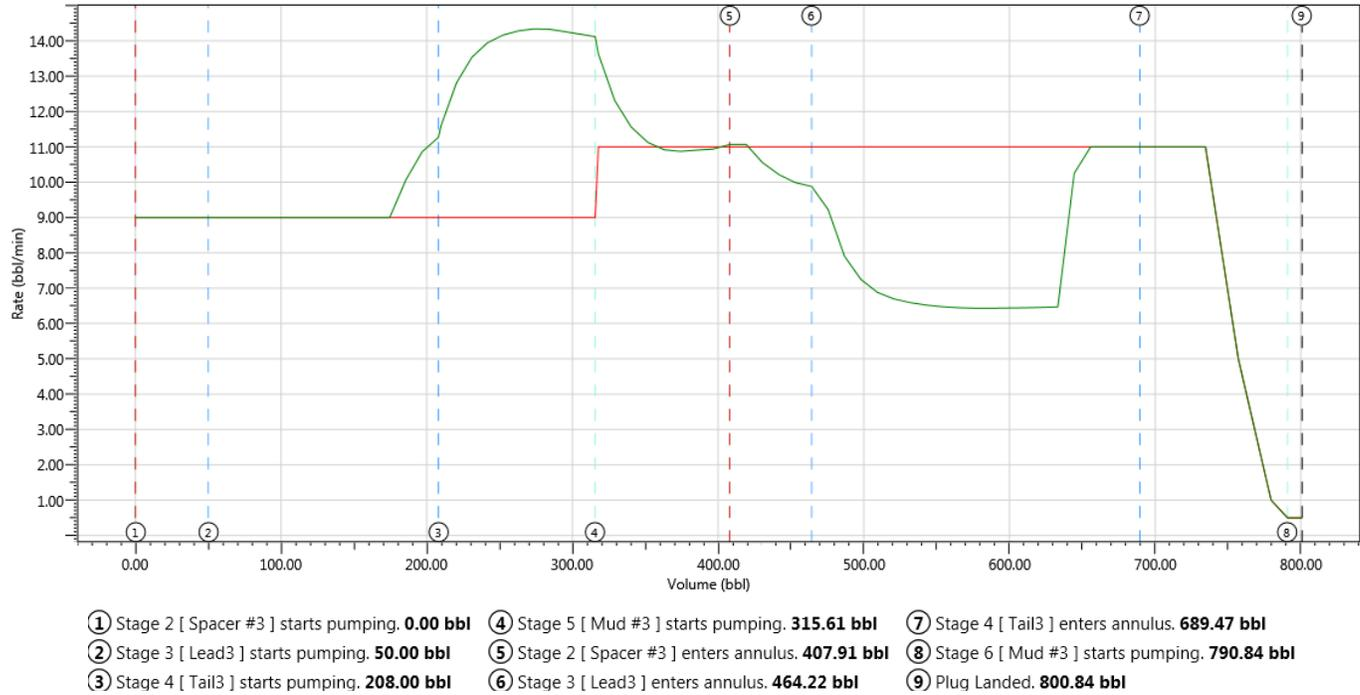
**Figure 10: The fluids pumping schedule for losses free design**
