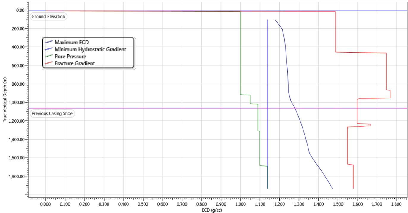
**Figure 7: The operation parameters for cement design when complete losses is recorded**
