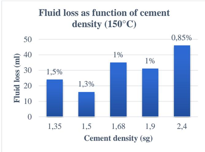
Figure 3: Fluid loss as function of the density of cement slurry. The percentage on the top of the column represents the concentration of micro-composite dry-equivalent by the weight of cement.
