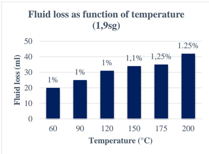
Figure 4: Fluid loss as function of temperature. The percentage on the top of the column represents the concentration of micro-composite dry-equivalent by the weight of cement.
