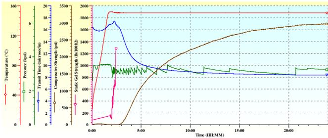
Figure 5: Static Gel Strength analyzer curve for 1.9sg cement slurry prepared with micro-composite.
