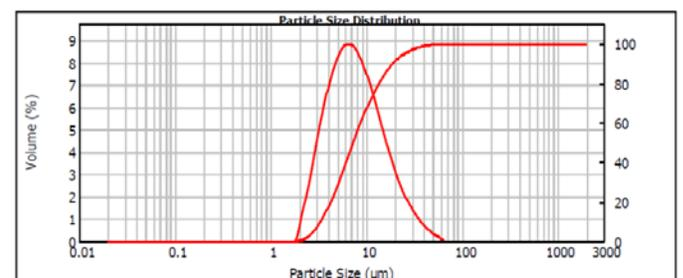
Figure 2: Light scattering particle size distribution of the micro-composite.
