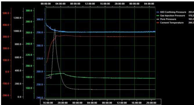
Figure 6: Gas Migration Analyzer for micro-composite 1.9sg cement slurry measured at 150°C.
