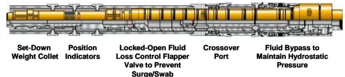
**Figure 2: Example of gravel pack tool**
