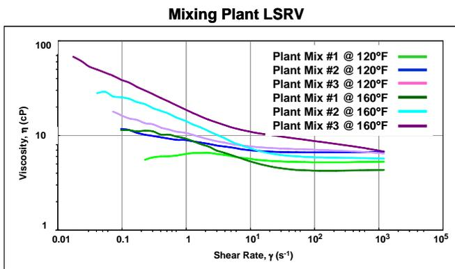
Figure 6: LSRV of plant batch mixes
