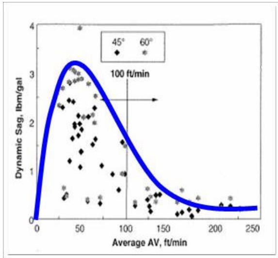
Figure 1: Average annular velocity vs measured dynamic barite sag (data scanned from Ref. 7).
