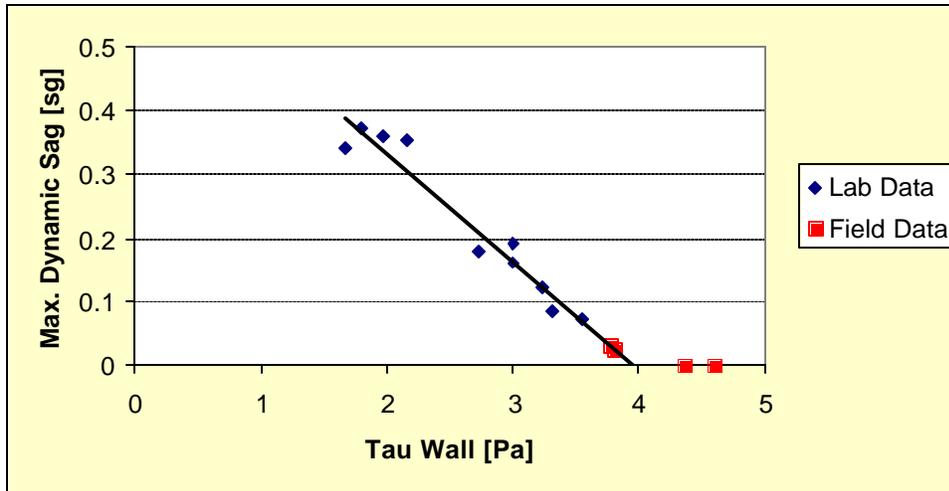
Figure 5: Dynamic barite sag predictions for selected new-generation invert emulsion field fluids.
