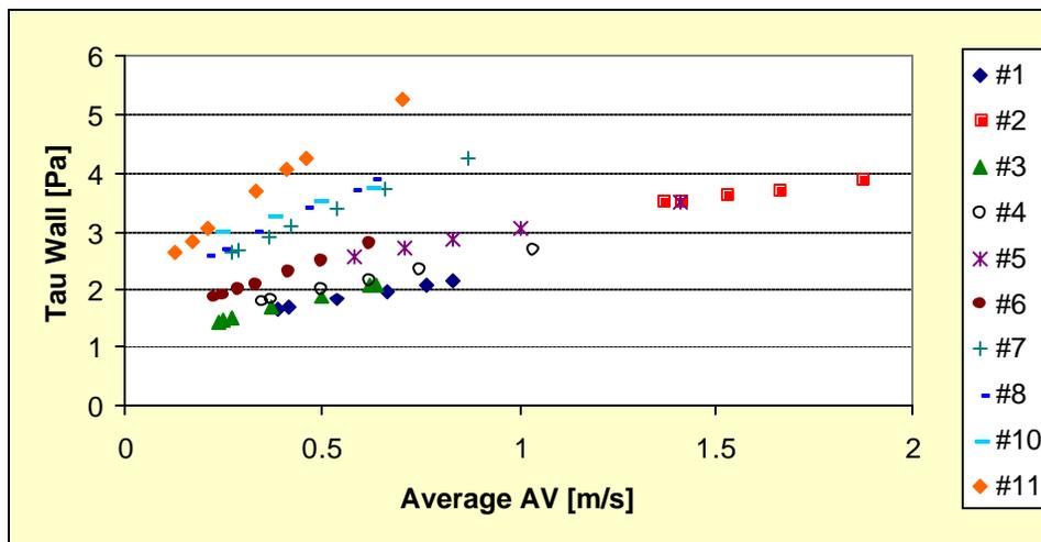
Figure 2: Average annular velocity vs. shear stress at the conduit wall by fluid number.
