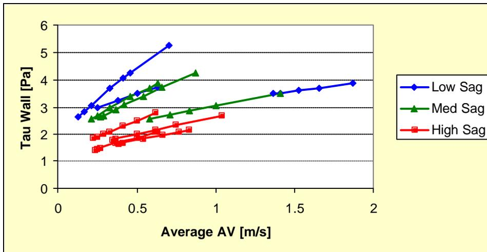
Figure 3: Average annular velocity vs. shear stress at the wall (data sorted by level of measured dynamic sag).
