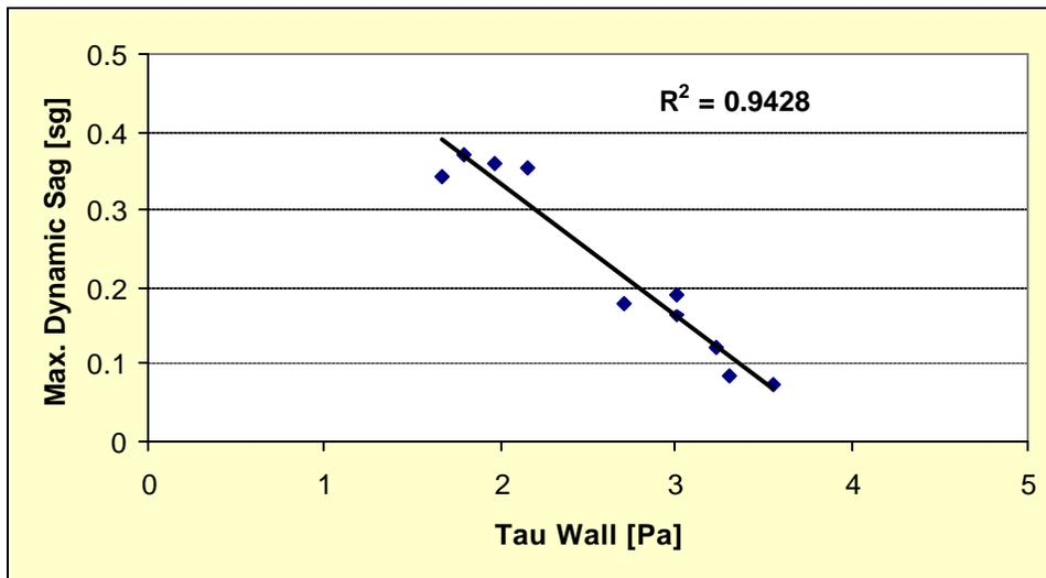
Figure 4: Shear stress at the wall vs. maximum predicted dynamic sag at an optimized average AV.
