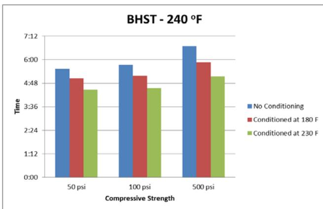
Figure 1 – Initial compressive strength at 240 °F
