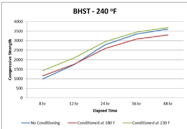
Figure 4 – 48 hour Strength Development at 240 °F
