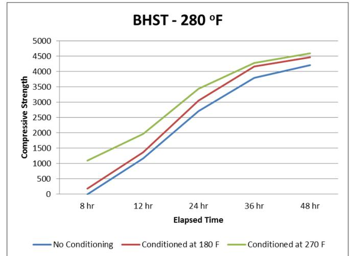
Figure 5 – 48 hour Strength Development at 280 °F
