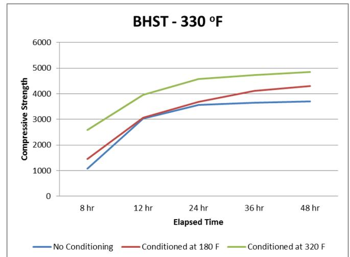
Figure 6 – 48 hour Strength Development at 330 °F
