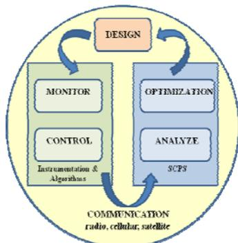
Figure 1 - Cycle for automation optimization, including Solids-Control Process Simulator (SCPS) management tool.
