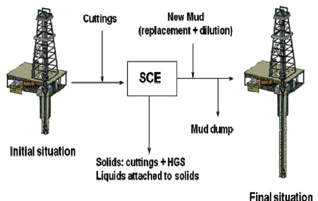
Figure 3 - Basic loop for a mud system.
