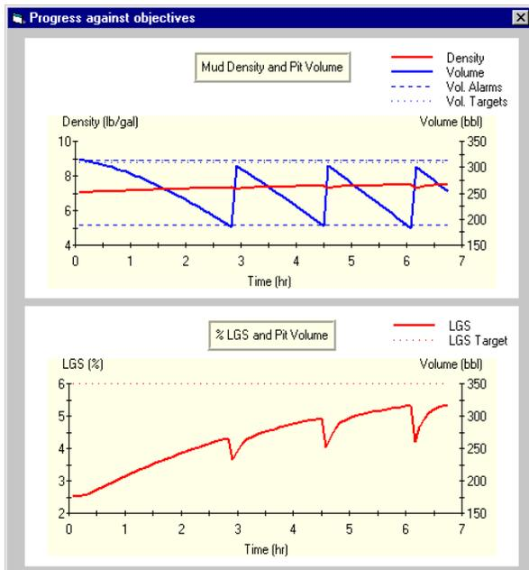
**Figure 7 - Examples of real-time corrective action plots for a mud system; correcting mud density, %LGS and pit volume.**
