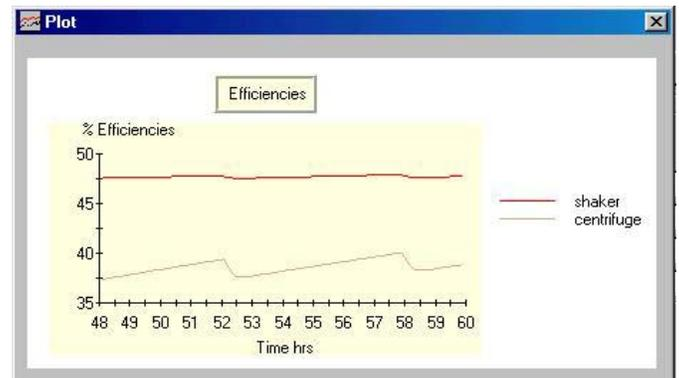
Figure 6 - Sample plot of shaker and centrifuge efficiency real-time data.
