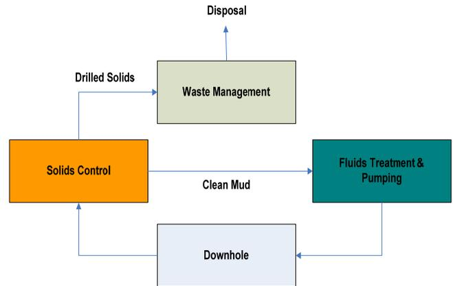
Figure 2 - Schematic of Wellbore Construction Fluids Domain
