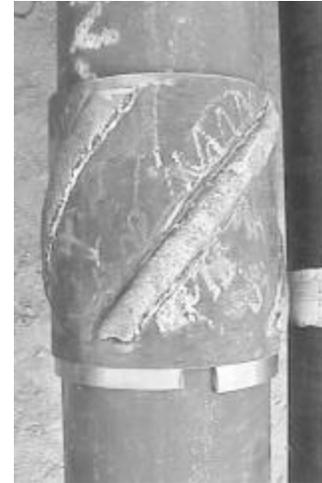
**Figure 3:** Shrink fit rigid centralizer.
