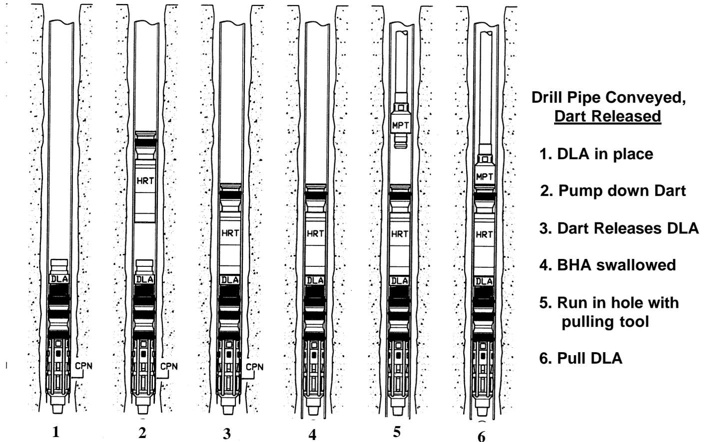
**Figure 11:** New generation dart released drill lock.
