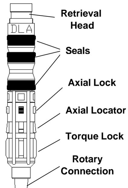
Figure 1: Drill Lock Assembly
