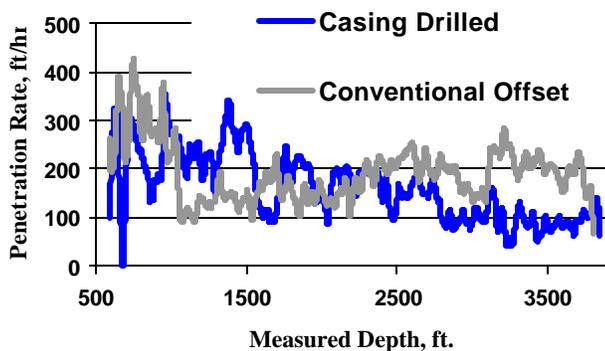
**Figure 6:** Instantaneous penetration rates.
