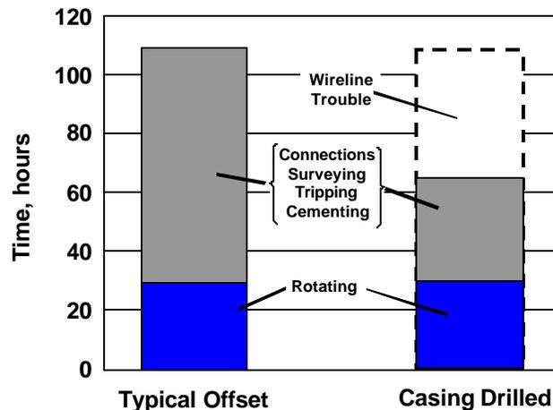
Figure 9: Comparison of conventional and Casing Drilled deep surface hole.
