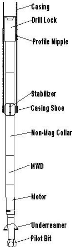
**Figure 2:** Casing Drilling system.
