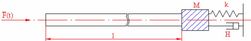
Figure 1, Drillstring model
