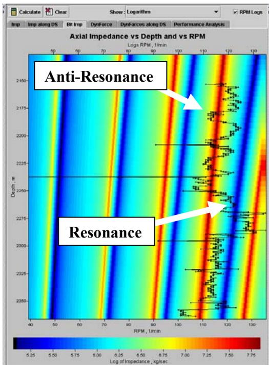
Figure 3, Mechanical Input Impedance at Bit Face
