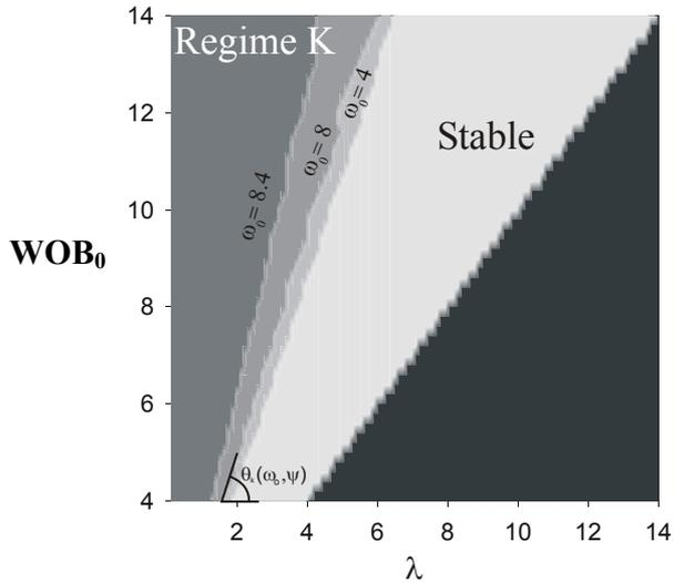
Figure 9, Parametric Stability Map
