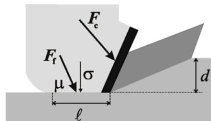
Figure 6, Frictional and Cutting Force Acting on a Cutter [9]
