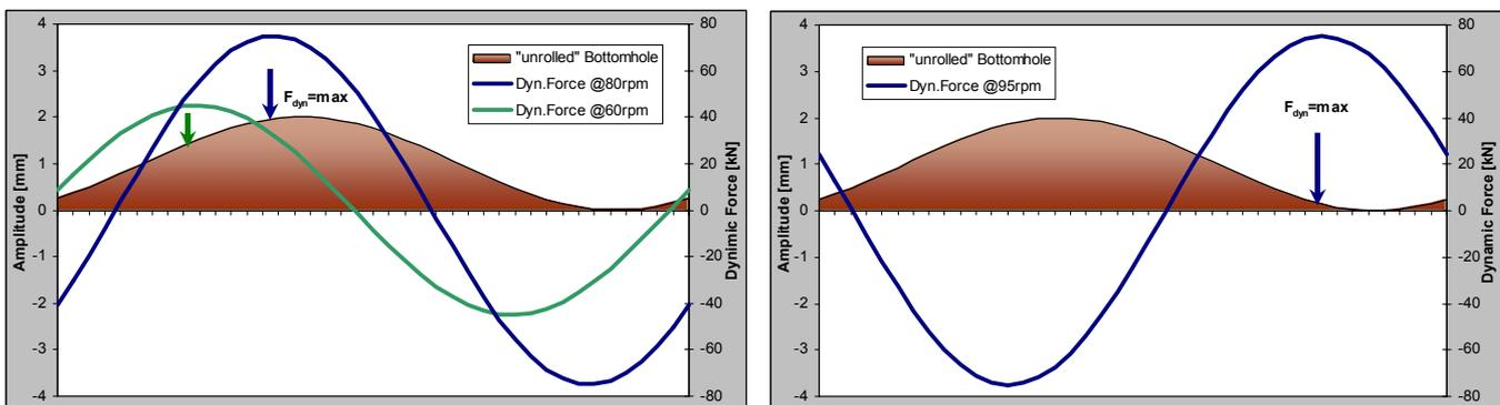
Figure 2a and 2b, Rock Destruction in dependence of Phase Shift
