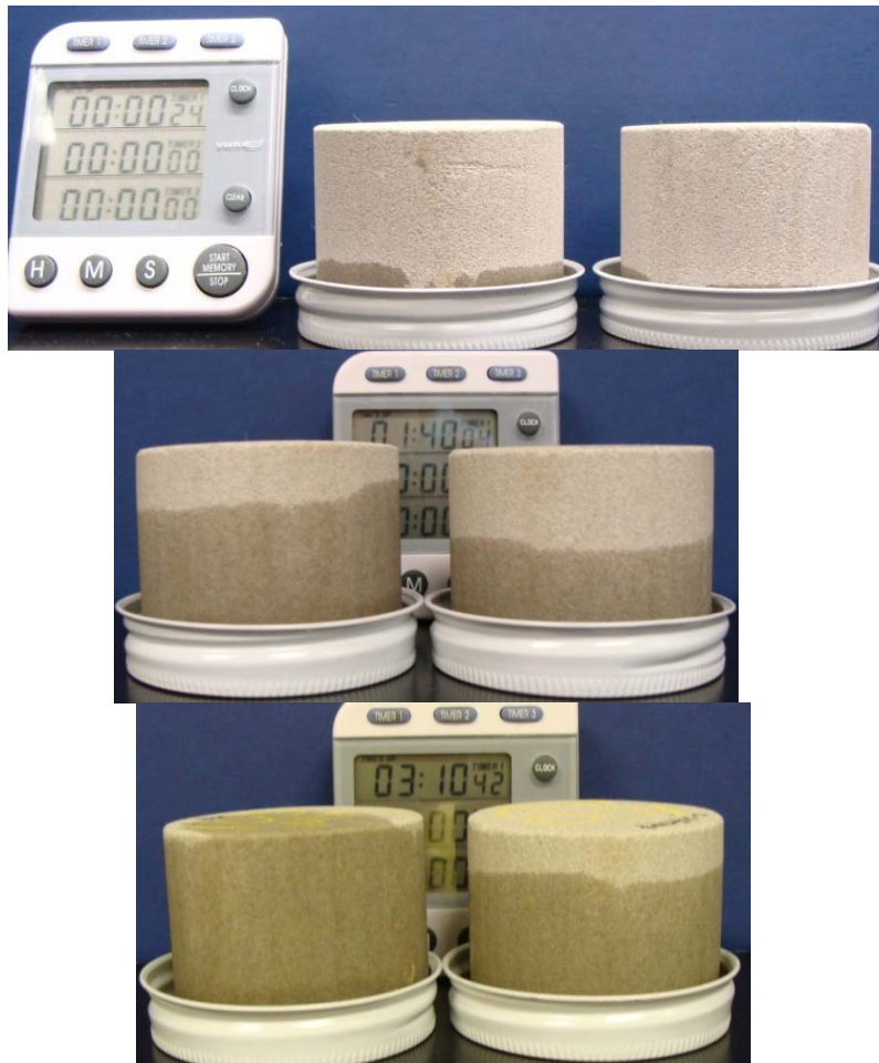
Fig. 4: Imbibition of brine into dry sandstone cores. Both cores are resting in 11.6-lb/gal \text{CaCl}_2 brine. The core on the left is untreated and the core on the right is treated with flow-back enhancer. Note imbibition of brine as time increases from top to bottom of photo sequence.
