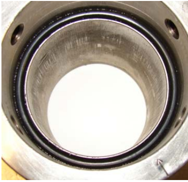
Fig. 3-1: Fann HTHP cell with FA0-00 disk.
