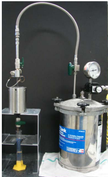
Fig. 3-3: Fann cell connected to air pressure charger.
