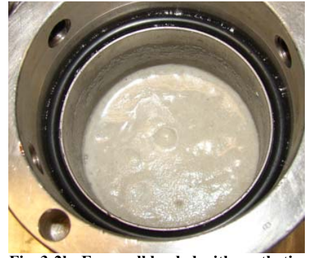
Fig. 3-2b: Fann cell loaded with synthetic formation and brine.
