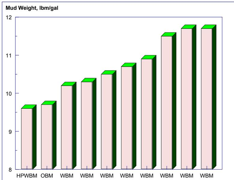
Figure 6 –Maximum mud weight at TD of 12 ¼” interval on South Texas well
