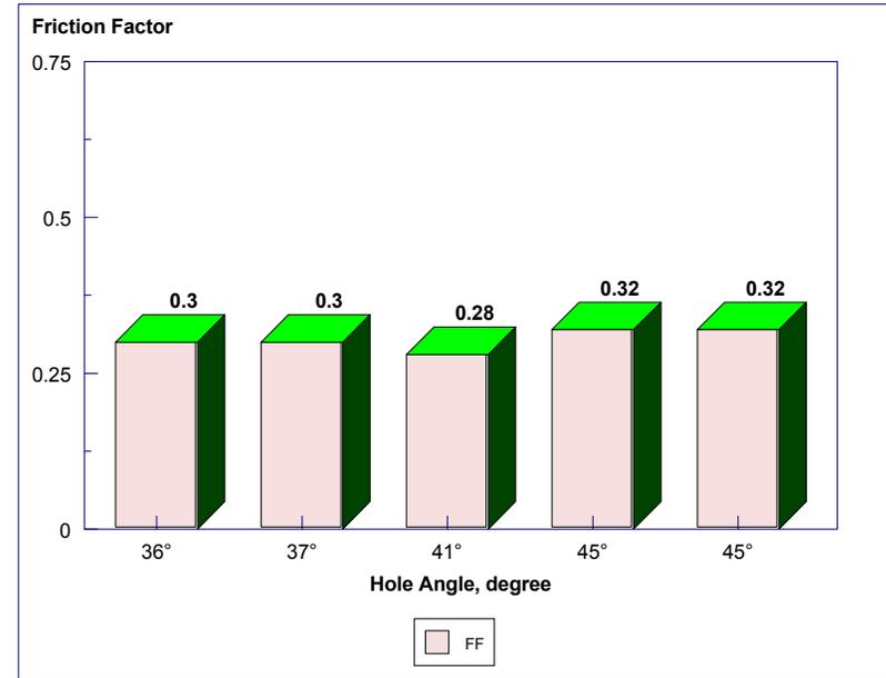
Figure 11 – Friction factors for HPWBM from GoM deepwater well
