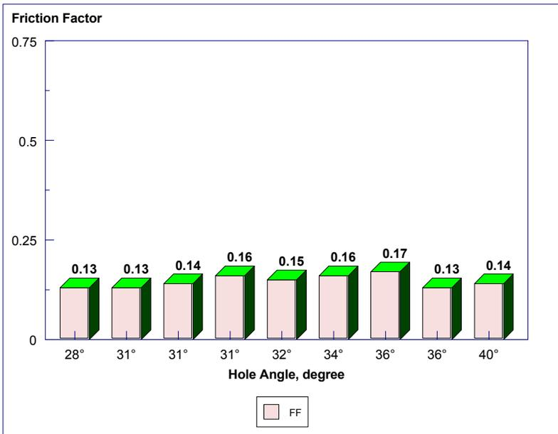
Figure 2 – Friction factors for HPWBM from onshore well
