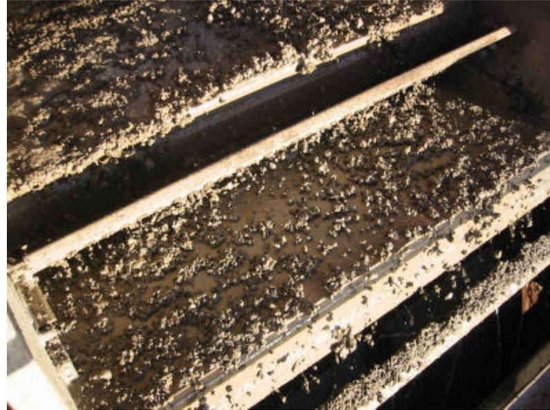
Figure 3 –Cuttings over 145 mesh screens and 175 feet/hour ROP- South Texas
