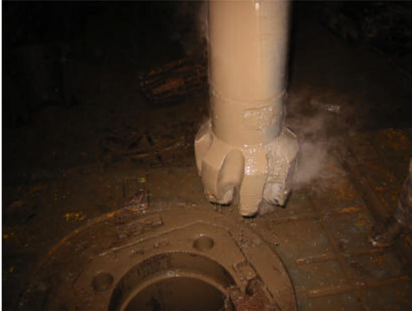
Figure 5 – PDC bit during trip with freshwater HPWBM in South Texas
