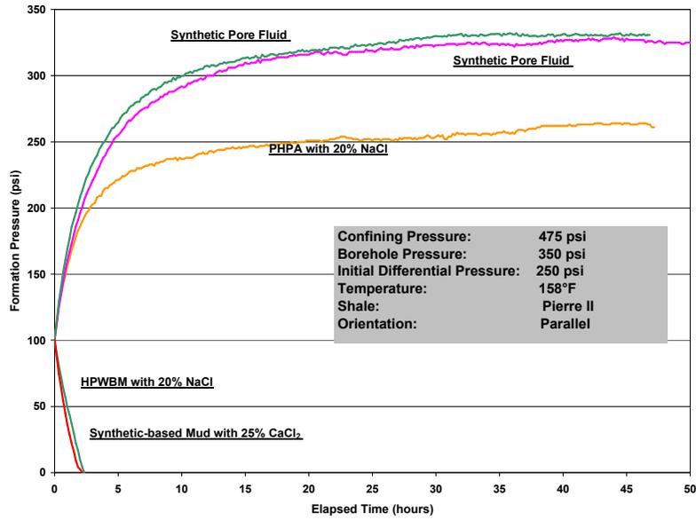
Figure 1 – PPT Tests comparing WBM, SBM and the HPWBM
