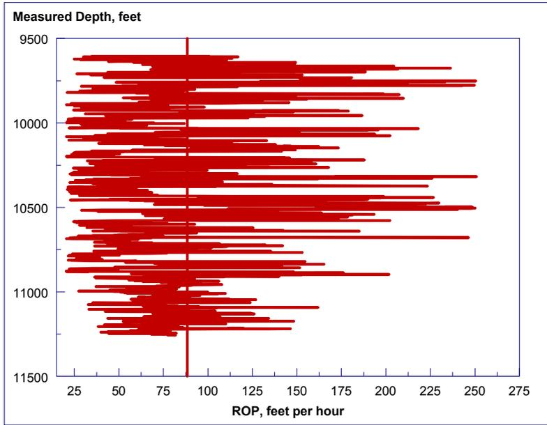
Figure 9 – Rates-of-penetration in 12 1/4” interval of GoM deepwater well
