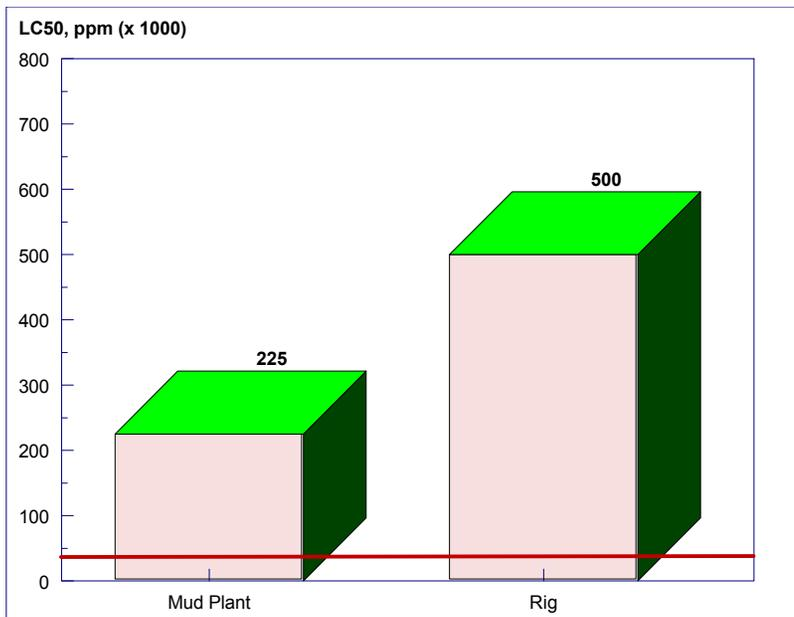
Figure 10 – US LC<sub>50</sub> values of HPWBM from GoM deepwater well
