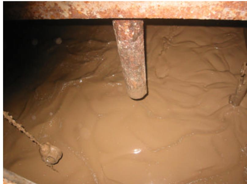
Figure 12 – HPWBM (20 % NaCl) in surface pits
