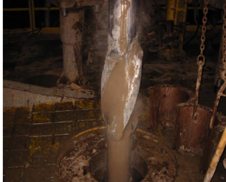
Figure 4 – Stabilizers during trip with freshwater HPWBM in South Texas
