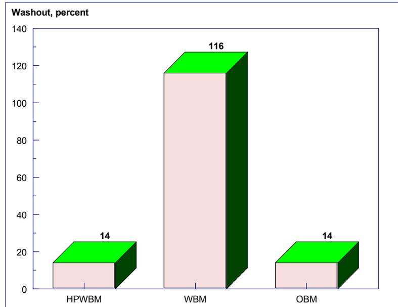
Figure 8 –Hole enlargement comparison in 12 ¼” interval on South Texas well
