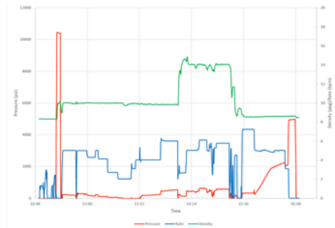
Figure 7 – Job log with WBS spacer system
