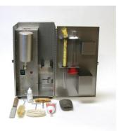
Figure 1 Retort distillation kit
