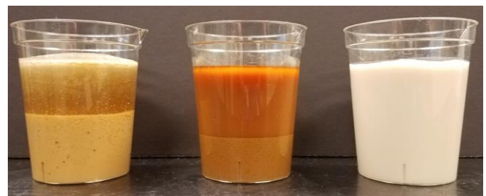
Figure 2. Unstable systems vs. stable system
