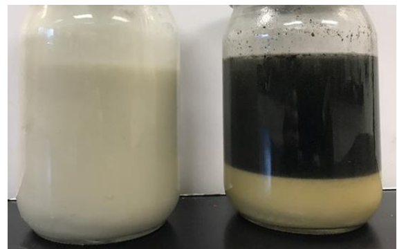
Figure 6. New HPHT RDF versus conventional brine-based system
