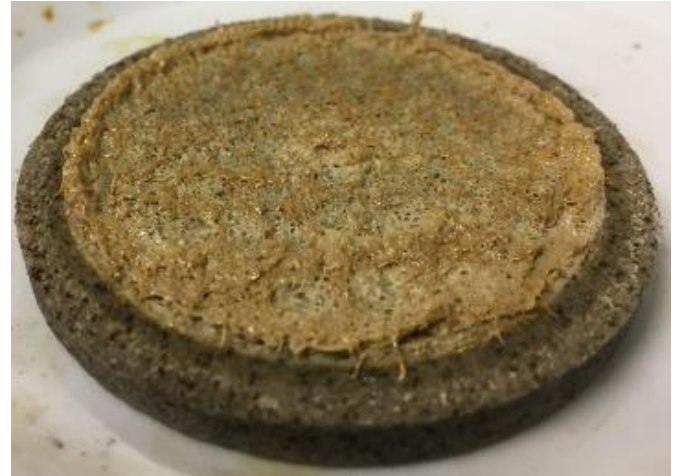
Figure 15. Disk after acid/acid precursor treatment
