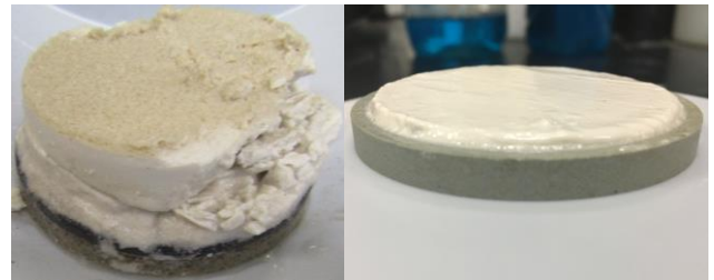
Figure 1. Thick filtercake vs. thin filtercake
