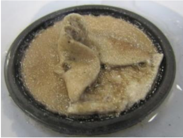
Figure 13. Disk after acidic breaker system treatment
