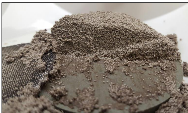
Figure 20- Partially Dissolved and Disperse Filtercake after breaker Treatment
