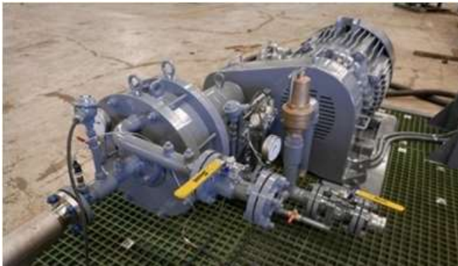
Figure 1 – High-shear, controlled-cavitation (HSCC) mixer.
