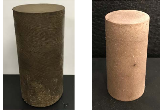
Figure 12 - Pictures of geopolymer hybrid samples containing {left} 20% SBM used in US horizontal well drilling operations and {right} 20% OBM used in offshore Thailand drilling operations.
