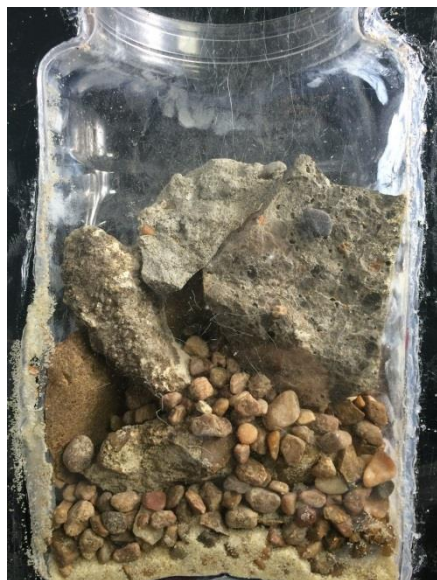
Fig. 2a – Simulation of a limestone formation with relatively large voids as well as loose fragments, pebbles and sand (left). A 10.7-lb/gal PBS system immediately after pouring into the plastic container (right).
