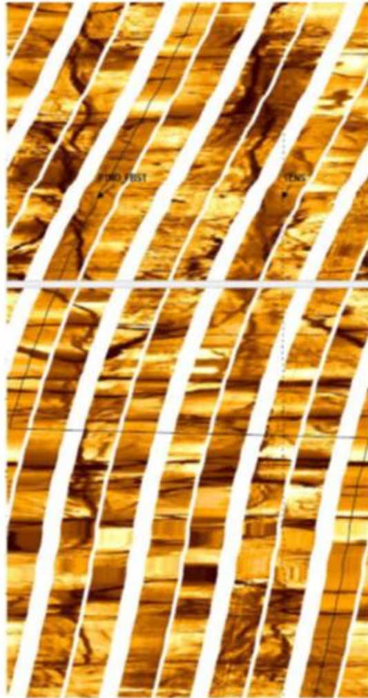
Fig. 9 – Selected section from the FMI run in Well A, 8 \frac{3}{4} -inch wellbore as run/processed after controlling losses.
