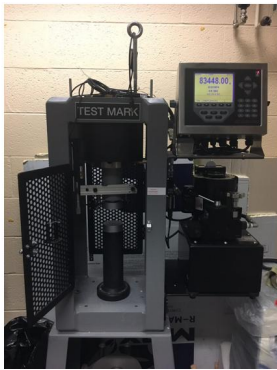
Figure 4. Certified crush test for UCS measurements
