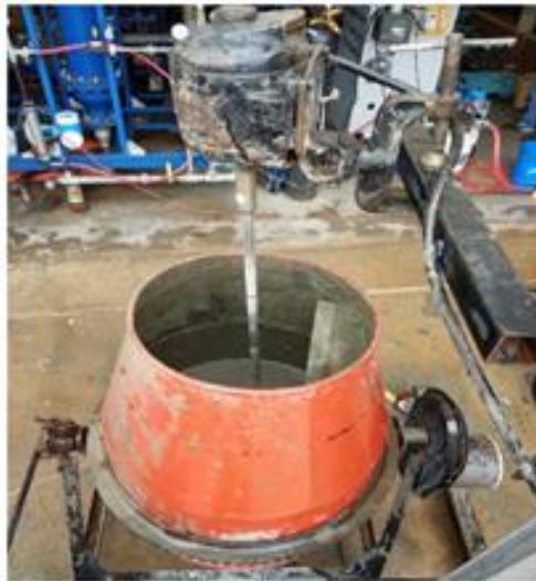
Figure 7: Drum mixer was used to prepare and mix cement slurry at low rpm
