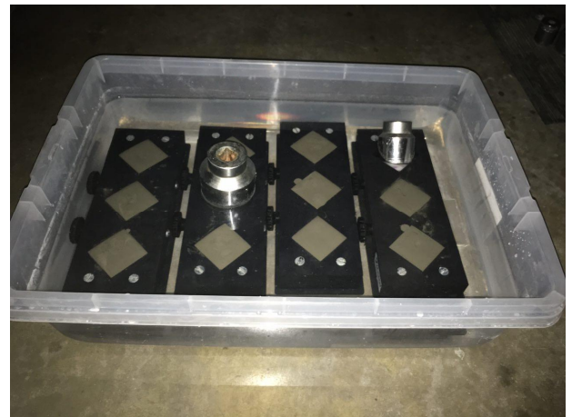
Figure 3. Cement specimens cured in water bath before being used for UCS testing
