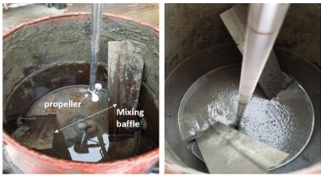
Figure 7: Drum mixer was used to prepare and mix cement slurry at low rpm
