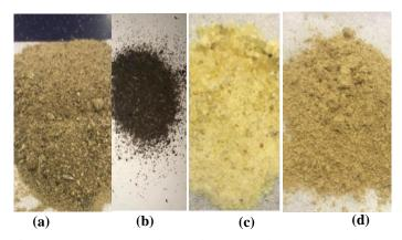
Figure 2. (a) Banana Peels Powder (BPP), (b) Banana Peels Ash (BPA), (c) Gum Arabic Powder (GAP), (d) Potato Peels Powder (PPP)
