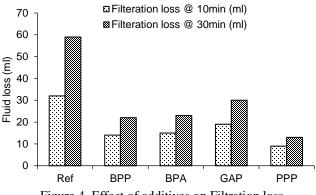
Figure 4. Effect of additives on Filtration loss
