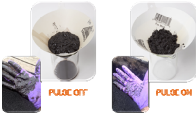
Fig. 6 —Cuttings from the Paint Filter Liquids Test, with and without the fluid and cuttings separator system.
