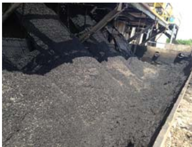
Fig. 3 —Dry cuttings in the bin below three shakers running the fluid and cuttings separator system.
