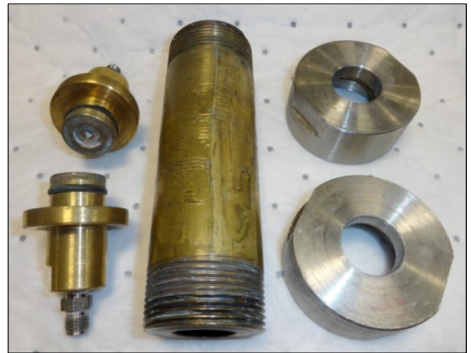
Fig. 1—Sandpack assembly used for testing.
