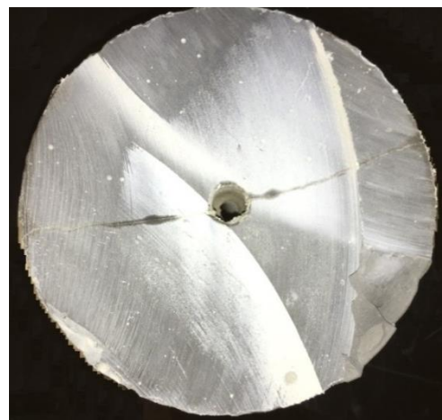
Figure 2. Symmetric and bi-wing fracture created around the wellbore for Test #7
