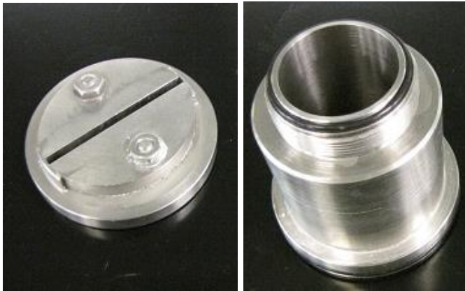
Fig. 3—The adjustable slot, shown face down (left) and the cell cap custom piece (right).
