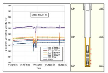
**Fig. 4.** Different points of interest are monitored in real time in addition to the ECD at the APWD's position. Five points of interest are monitored (i.e., a week sand below the casing shoe).
