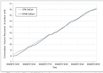
**Fig. 11.** The RTHM software calculates the cumulative volume recovered at surface, this can be compared vs the actual volume in order to determine if cuttings are remaining in the well or not.
