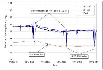
**Fig. 3.** The RTHM software performs ESD calculations in real time, and the results are compared every connection against the APWD.
