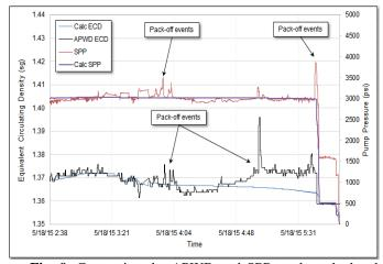
**Fig. 9.** Comparing the APWD and SPP vs the calculated values, can help to avoid hole cleaning problems that lead in NPT.
