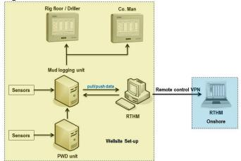
**Fig. 1.** Basic configuration for wellsite communications. Calculations are performed at the wellsite and managed onshore.
