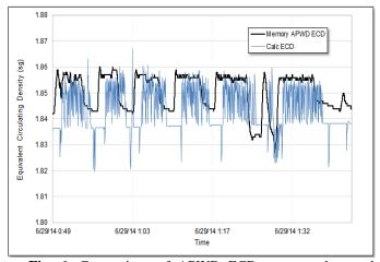
**Fig. 6.** Comparison of APWD ECD memory data and RHTM software while tripping in the hole after recovering the APWD memory data.
