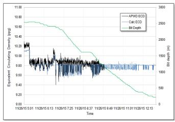
**Fig. 5.** Comparison of APWD ECD memory data and RHTM software while pulling out of the hole after the APWD memory data is recovered.
