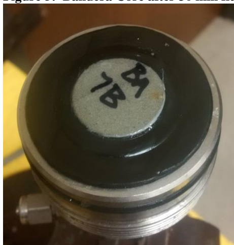
Figure 5: Bandera Core after 30 min fluid loss at 100 psi
