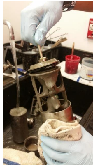
Figure 6. Gelling around Paddle for slurries tested at high temperature without addition of superplasticizer
