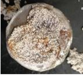
Figure 9- Core plug after return permeability test showing filtercake completely dissolved after 4 days breaker soak.
