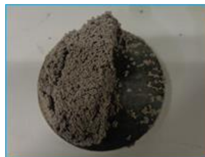
Figure 8- Aloxite disk after a 5-day break soak; no filtercake residue left on the disk.
