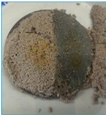
Figure 6- Aloxite disk after a 2-day break soak-no filtercake residue left on the disk.
