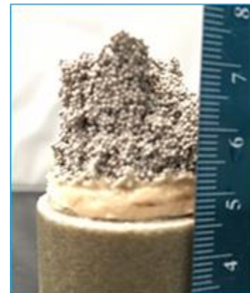
Figure 7- Core plug after return permeability test showing filtercake not dissolved after a 2-day breaker soak.
