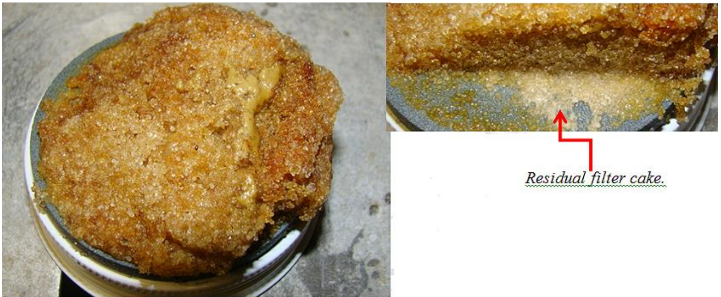
Figure 8 – Texture and high-magnification views of filtercake and gravel from the Breaker #2 test.
