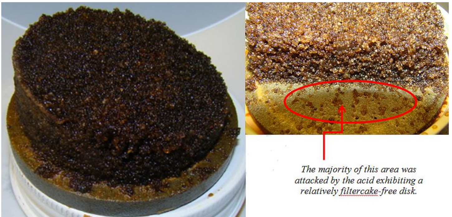
Figure 9 – Texture and high-magnification views of filtercake and gravel from Breaker #3 test. Note the absence of residual filtercake.
