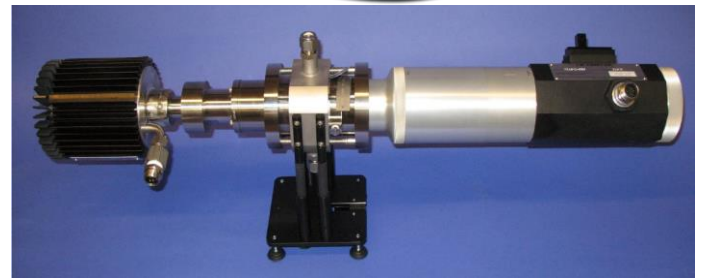
Figure 11 – PSA systems for real-time, automated monitoring in the field: (top) MT G600 Ex (image courtesy Mettler Toledo; (bottom) Canty In-Line Drilling Fluid System (image courtesy JM Canty).
