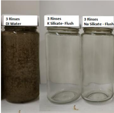
Figure 1: flush efficiency jar test
