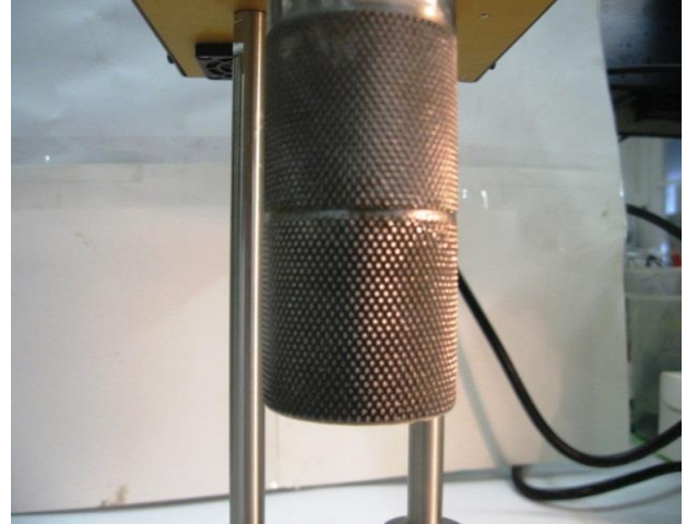
Figure 2b: Rotor after 5 minute flush in K silicate solution
