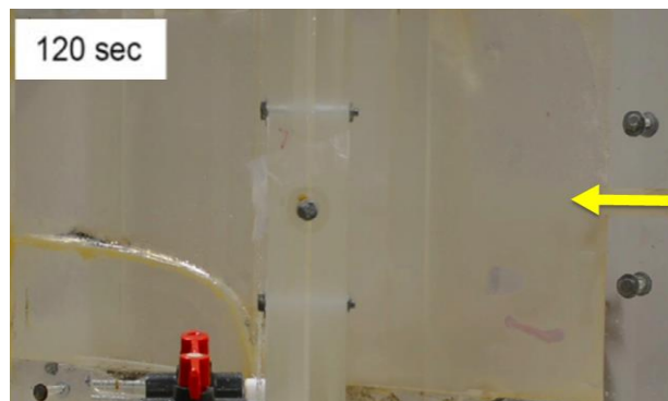
Figure 6. Slot Test of a suspension of 2.00 gpt LG slurry with 2.00 ppa showing no proppant settling.
