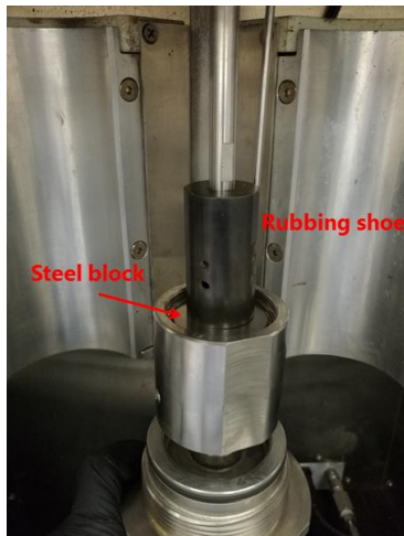
Figure 4: Rubbing shoe and steel block set-up inside the sample cell.
