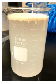
Figure 7: Cheesing of Lubricant A in 10% \text{CaCl}_2 brine.
