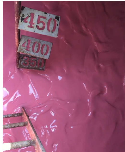
Figure 3. The direct emulsion system mixed in tanks prior to drilling.
