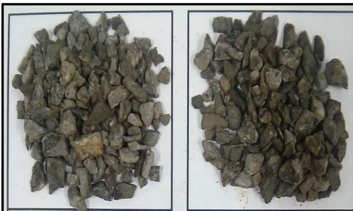
Figure 5: Shale cuttings after the shale recovery tests
