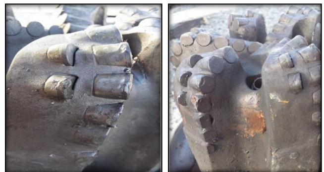
Fig.12. Used bit POOH with worn cutters mainly in the shoulder area indicating a good run for this bit.
