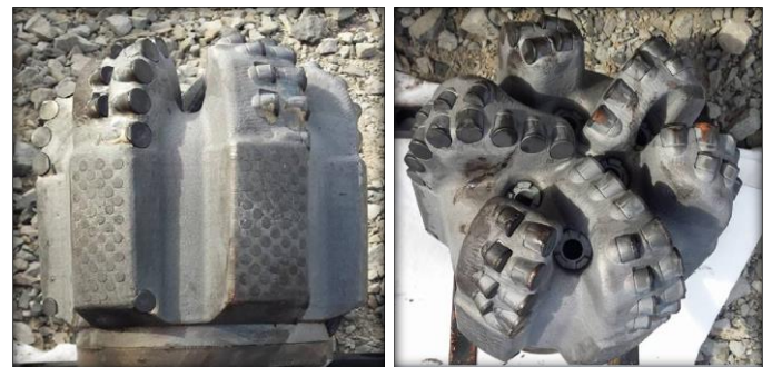
Fig.14. PDC pulled out of the hole after drilling 7,600ft of formation was in a good, repairable condition.
