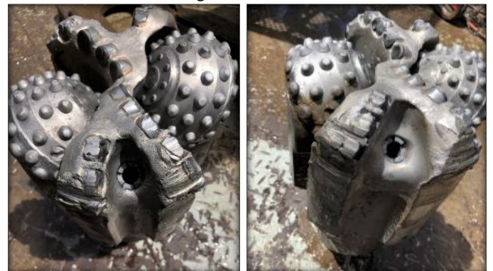
Fig.10: Worn PDC cutters on the shoulder and gauge area of this hybrid drill bit when examined at surface after POOH.
