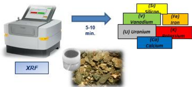
Fig.04. High precision X-Ray Fluorescence technique used on-site to track the elemental composition of the drilled cuttings.
