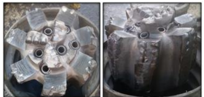
Fig.08: Worn PDC cutters on the shoulder and gauge area of this hybrid drill bit when examined at surface after POOH.
