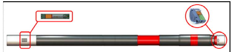
Fig. 3: Mud Motor with Embedded Sensors in Bit Box and Top Sub (excerpted from AADE-17-NTCE-077)
