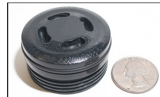
Fig. 6: Sensor in a “hockey puck” shaped package
