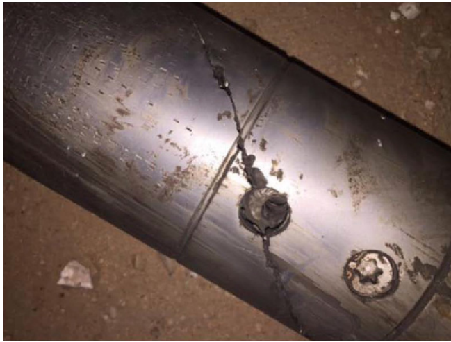
Fig. 1: 45° collar cracking (third-party tool) due to severe HFTO (excerpted from SPE-187173)
