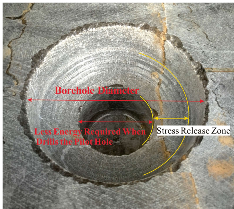
Fig.6 Actual hole drilled by WOB Self-Adjusting Dual-Diameter Bit
