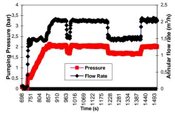
Figure 8 – Pumping pressure and annular flow rate x time – Geometry 1
