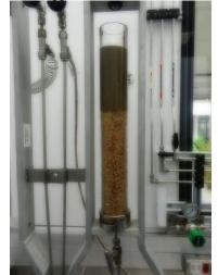
Figure 1 – Static filtration an unconsolidated bed
