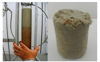
Figure 6 – Static filtration test in high permeability limestone bed
