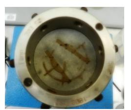
Figure 12 – Static filtration in fractured porous media – Pill D
