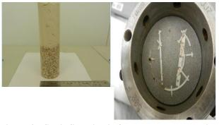
Figure 4 – Static filtration in fractured porous media – Fluid A
