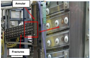
Figure 3 – Fracture flow simulator with 2, 5 and 10 mm aperture
