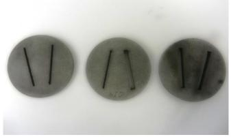
Figure 2 – Porous media of 1 and 2 mm apertures
