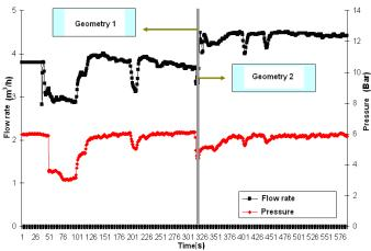
Figure 13 – Pressure and Flow rate profile at the Fracture Flow Simulator tests – Pill D
