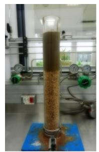
Figure 11 – Static filtration test on limestone bed – Pill D
