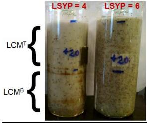
Figure 2: Suspension of 850-1000 µm LCM particles (ground walnut particles) in two drilling fluids (fluid B and fluid C) with variation in LSYP (mud weight= 9.0 ppg).
