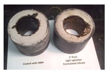
Figure 3c: Glass G Cement Plug & extrusion test
