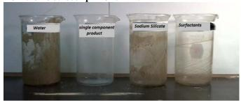
Figure #2: Flush Volume Efficiency using OBM from field
