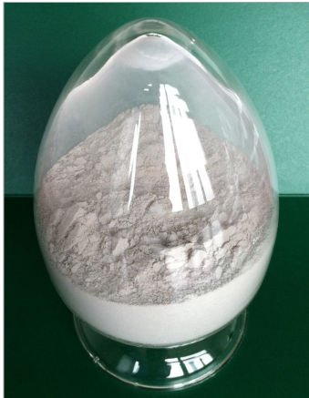
Figure 13. Optimized fracture sealing formulation for ultralow spurt losses.
