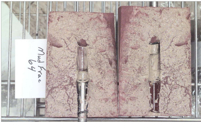
Figure 3. Split red sandstone core specimen.
