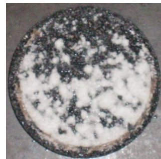
Figure 4 Formulation J before and after cleanup with Soltrol 170 at 250°F for 2 hours
