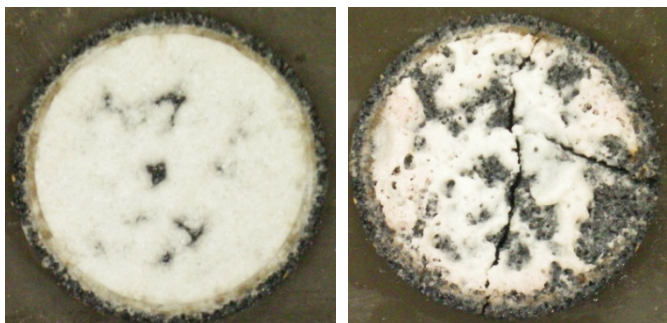
Figure 6 Formulation K before and after cleanup with Diesel at 250°F for 2 hours
