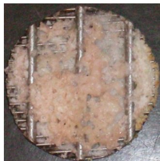
Figure 9 Formulation O after cleanup with Diesel at 250°F for 2 hours
