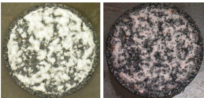
Figure 7 Formulation M before and after cleanup with Diesel at 250°F for 2 hours
