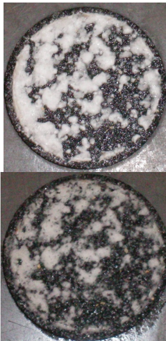
Figure 1 Formulation K before and after cleanup with Soltrol 170 at 250°F for 2 hours
