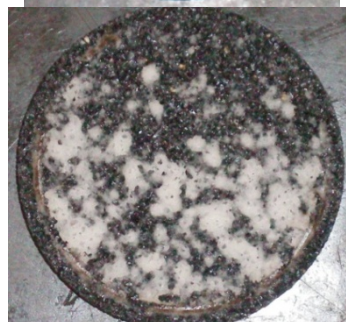
Figure 5 Formulation L before and after cleanup with Soltrol 170 at 250°F for 2 hours
