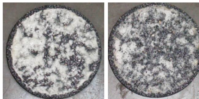
Figure 4 Formulation J before and after cleanup with Soltrol 170 at 250°F for 2 hours
