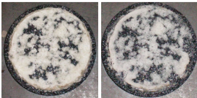
Figure 2 Formulation M before and after cleanup with Soltrol 170 at 250°F for 2 hours
