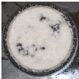
Figure 2 Formulation M before and after cleanup with Soltrol 170 at 250°F for 2 hours
