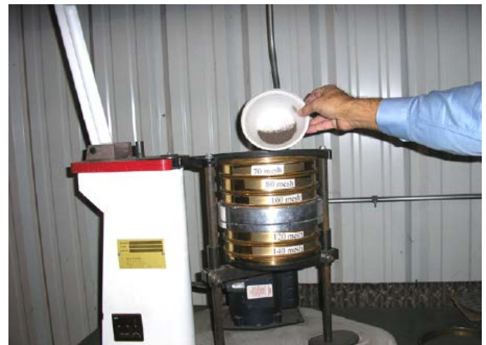
Figure 7 Test screen mounted between ASTM test sieves Image courtesy of Derrick Equipment Company
