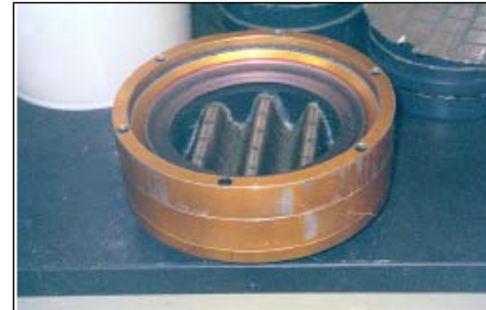
Figure 6 Test screen mounted in screen holder Image courtesy of Derrick Equipment Company
