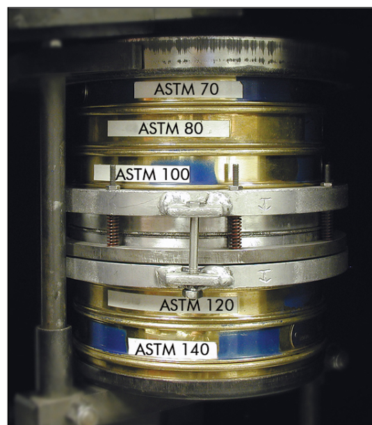
Figure 3. API RP 13C screen designation testing apparatus. Image courtesy of Derrick Equipment Company
