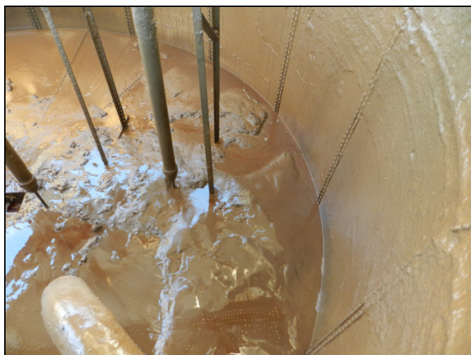
Figure 9: Oil-based mud residue settled in the mixing tank. Areas inside the tank have large sediment deposits accumulated over a period of time.
