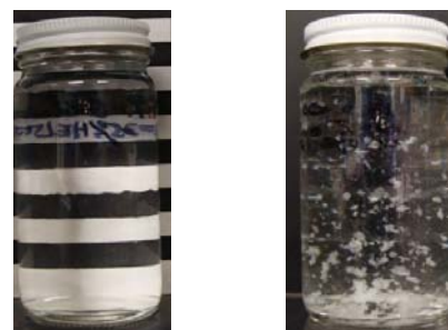
Fig. 4 – CaCl 2 brines containing both lubricant and drag reducer. Note that the combination on the left is soluble/dispersible in brine; and a different combination on the right is not dispersible in brine and shows “cheesing”.
